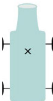
1. Cut a drinking straw into two pieces as long as the water bottle is wide. Use strips of tape to attach them to the bottle - one near the front and one near the back. The axles for the wheels will run through these straws, so line them up carefully so the wheels won't be crooked.
