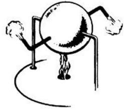
The jet engine of today operates according to this same basic principle. Jet engines contain three common components: the compressor, the combustor, and the turbine. To this basic engine, other components may be added, including:
